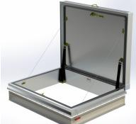
Three inches of polyisocyanurate insulation provide an R-value of 20-plus in both the cover and curb and a special cover gasket minimizes air leakage.
