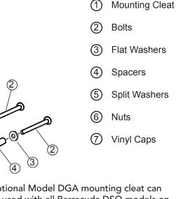
Optional Model DGA mounting cleat can be used with all Barracuda DSO models on doors with push bar locks or windows/side lights if glass breakage is a concern.
