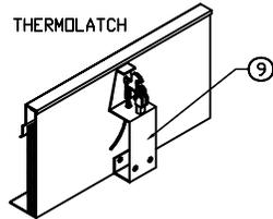
1. THERMOLATCH MECHANISM - COVERS WILL OPERATE ONLY WHEN ACTIVATED
